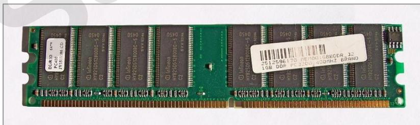
So RAM is volatile, meaning that its contents will be lost as soon as there is an interruption to power. RAM is also constantly changing with new contents flowing through on a regular basis.
