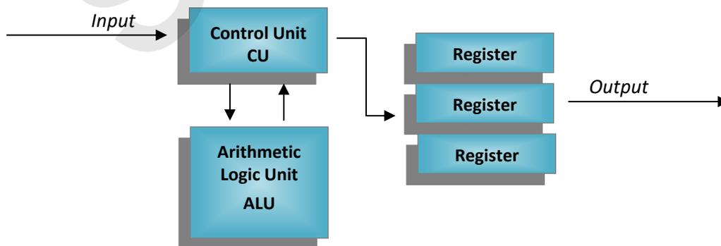
The **Control Unit** receives instructions and then assigns the task to the **Arithmetic Logic Unit**. Virtually all tasks involve arithmetic such as adding, subtracting, multiplying, and dividing, or logical operations such as "and", "or", and "not". This combination of arithmetic and logic allows the computer to perform very simple all the way through to extremely complex operations.
